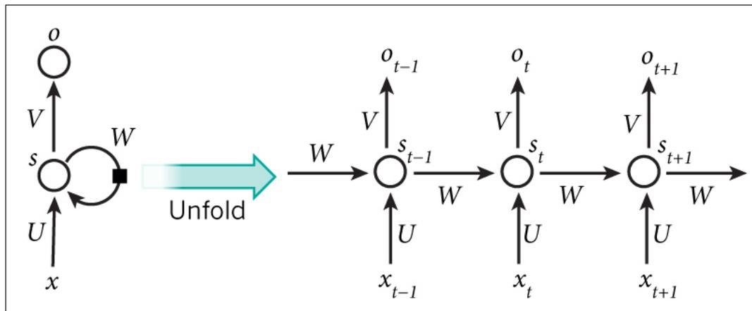
Figure 1: Unfolding of Recurrent Neural Network involved in Forward Computation
